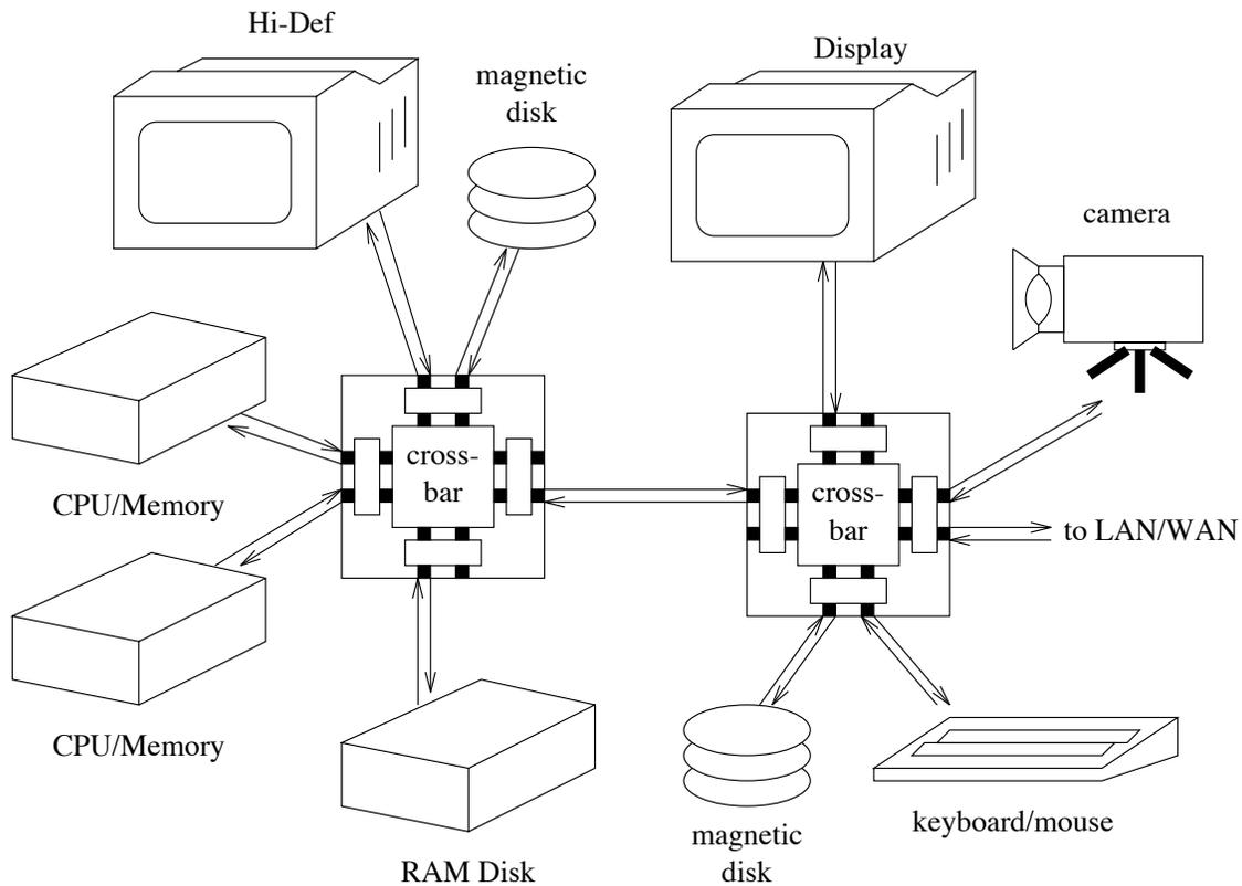
**Figure 1: Netstation Architecture**
