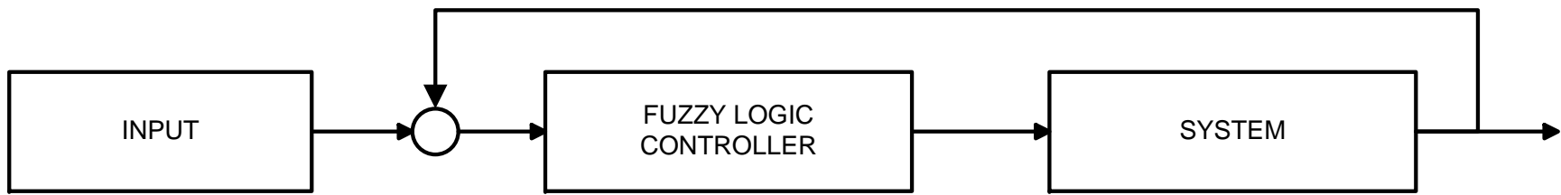
“Regular” Fuzzy Logic Control system
